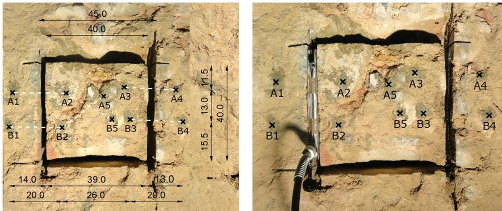
**Figure 12.** Shear flat-jack test setup and gage point's position (dimensions in cm).
