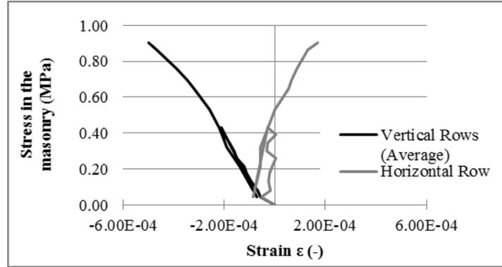
**Figure 4.** Relation between stress in the masonry and vertical and horizontal strains.
