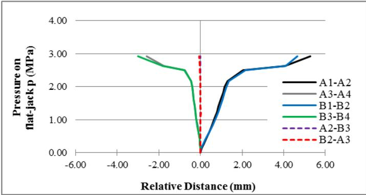
**Figure 10.** Loading cycle with a vertical pressure of 0.60 MPa.
