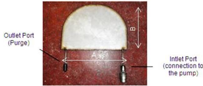
**Figure 1.** Semi-circular flat-jack with (A) 34.5 cm and (B) 25.5 cm.
