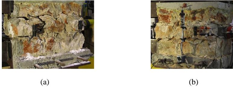
**Figure 2.4.** Collapse of masonry specimens: (a) specimen T1 and (b) specimen T7
