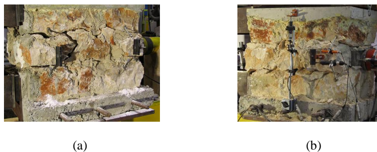
Figure 3.7. Collapse of masonry specimens: (a) specimen T1 and (b) specimen T7
