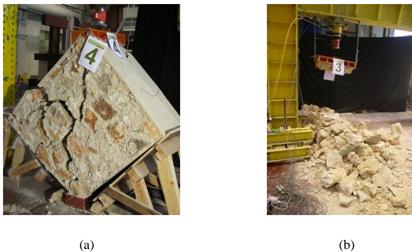
Figure 2.4. Collapse of masonry specimens: (a) specimen W4 and (b) specimen W3
