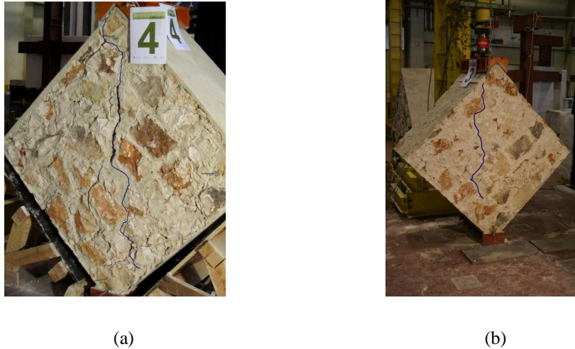
Figure 2.3. Main crack at the middle of the specimens: (a) specimen W4 and (b) specimen W3
