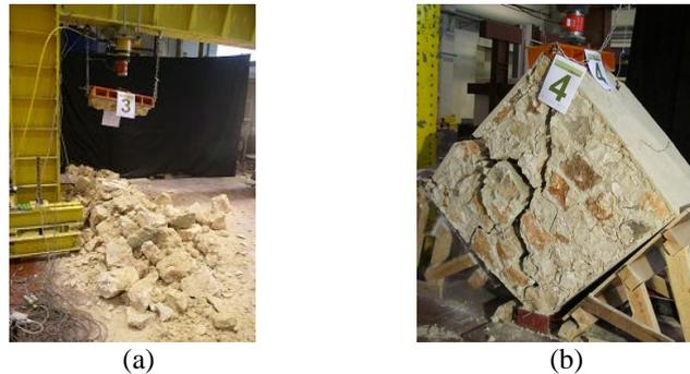
**Fig. 6** Collapse of masonry specimens: (a) specimen W3 and (b) specimen W4
