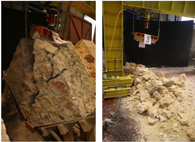
(a) Specimen W1 made with hydraulic mortar (b) Specimen W2 made with air lime mortar
