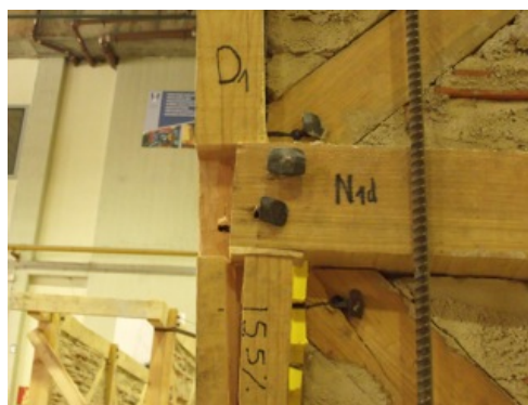
Figure 4-28: Failure by pull out of nails at connection N1d at a displacement of plus 90 mm
