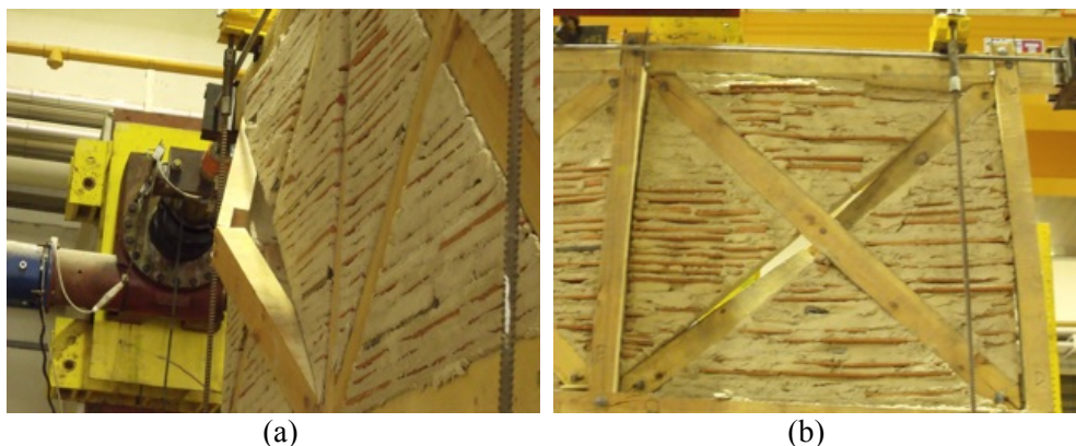
Figure 4-39: Failure by buckling of the upper left module diagonal, displacement of 90 mm in the positive direction of loading: (a) side, (b) back
