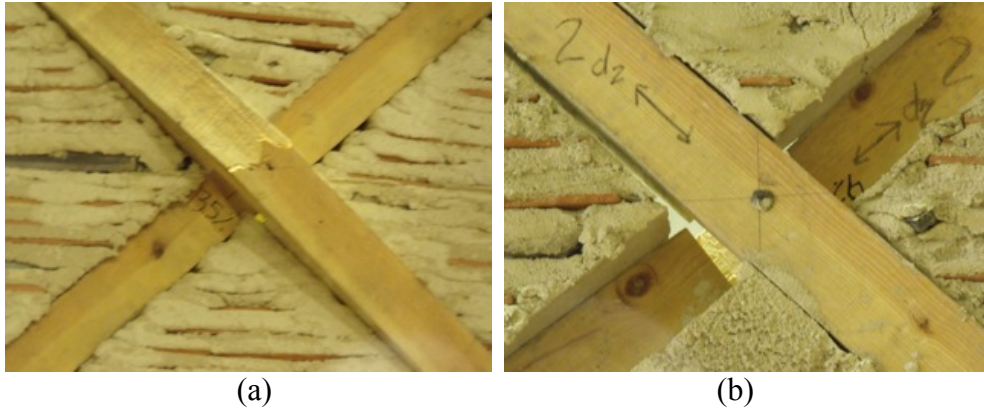
Figure 4-35: Buckling of diagonal in the upper module: (a) front; (b) back
