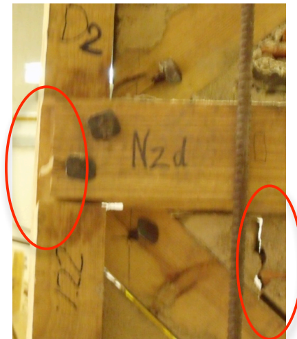
Figure 5-10: Pull-out of nails leading to gaps and residual displacements; masonry crack
