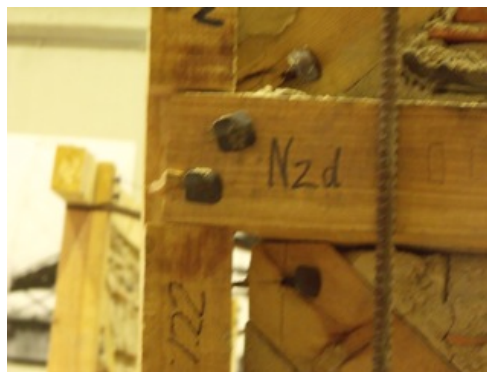
Figure 4-34: Behaviour of the connection N2d with almost pull out of nails
