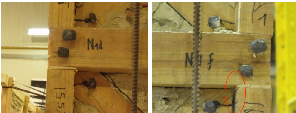
Figure 4-30: Detailing of the connections at a loading of minus 60 mm (from the left to the right)
