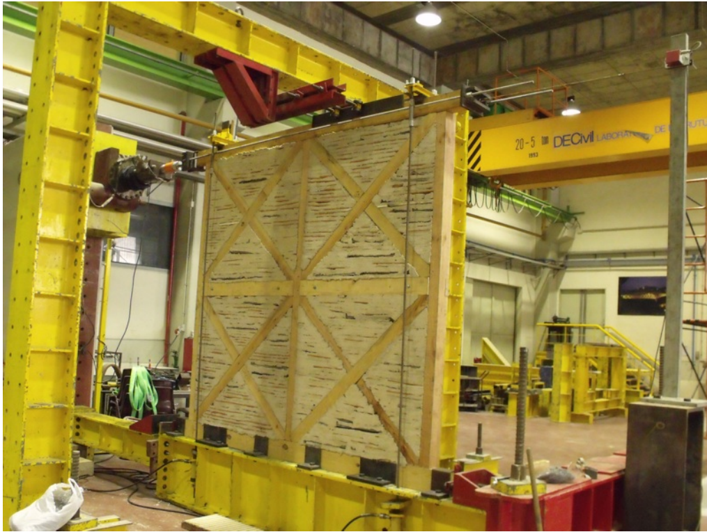
Figure 4-21: Final layout of the experiment with load cell, LVDT and jacks
