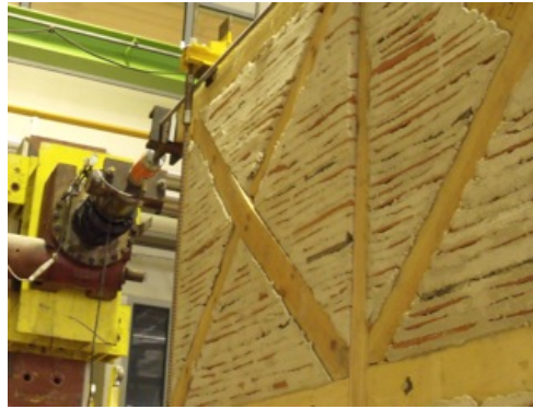
Figure 4-38: Initial out of plane instability of the upper left module, displacement of 60 mm in the positive direction of loading
