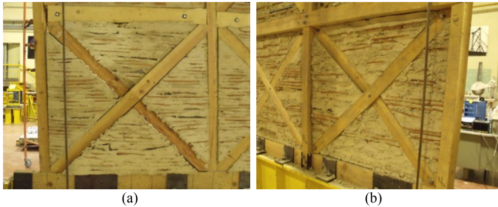
Figure 4-40: Failure of diagonal of lower left module: (a) front, (b) back; at displacement of 90 mm in the negative direction of loading
