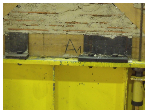
Figure 4-17: Steel shaped omegas to tighten the lower wood beam (brown) to the horizontal reaction beam (yellow)
