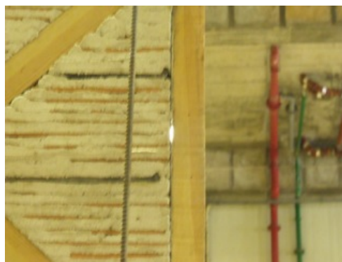
Figure 4-37: Detachment of the masonry panel from the wood truss
