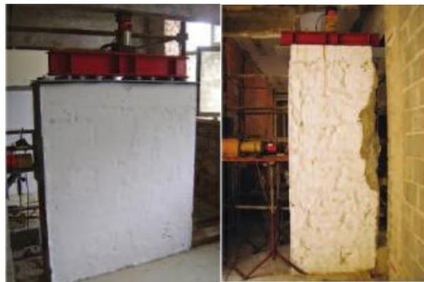
Figure 16 - General view of the two experimental models, voided concrete block and stonemasonry walls
