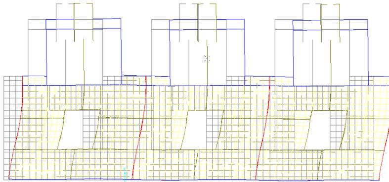
Figure 36 - The first vibration mode of the model.
