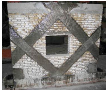
Fig. 17 Wall to be tested in-plane, strengthened with GFRP [Kabir et al, 2012]
