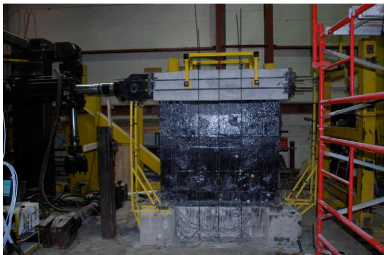
Fig. 16 Wall to be tested in-plane of brick masonry, strengthened with CFRP [Arifuzzaman and Saatcioglu, 2012]
