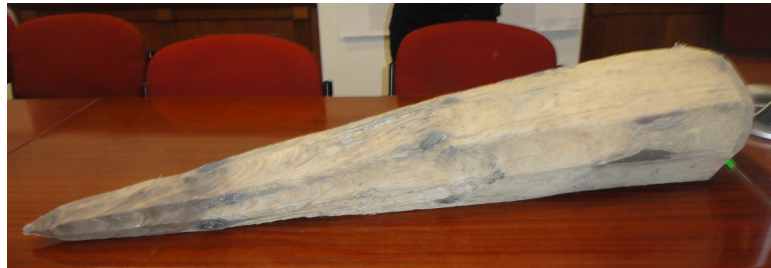
Figure 26 – Timber pile from a 'pombalino' building: experience has demonstrated that these timber piles are closer to 1 m length rather than 6 m.
