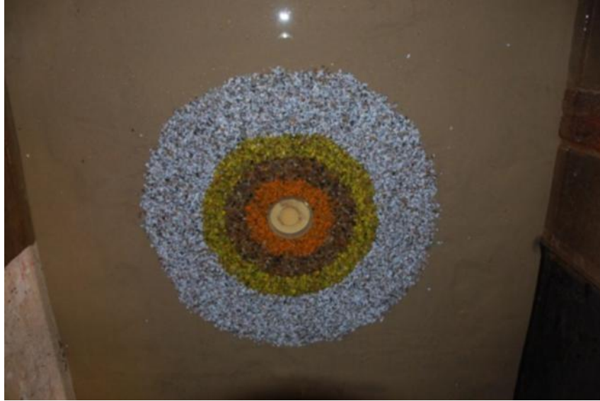
Figure 4.9 - Concentric configuration of the coloured rings around the monopile base, without the monopile.
