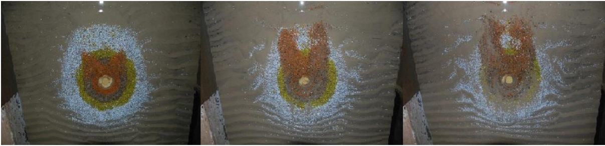
Figure 4.32 – Evolution of the V-shape form registered during s1_005: left – after 1000 waves, middle – after 3000 waves, right – after 5000 waves. Flow direction from the bottom to the top.
