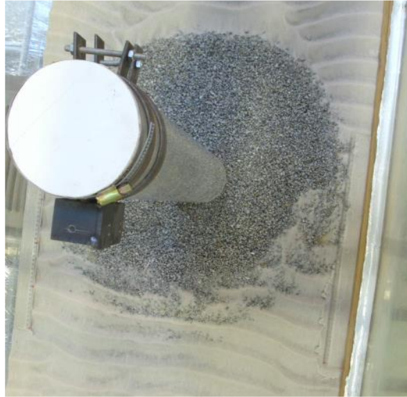
Figure 4.52 – Monopile and scour protection models after a test.
