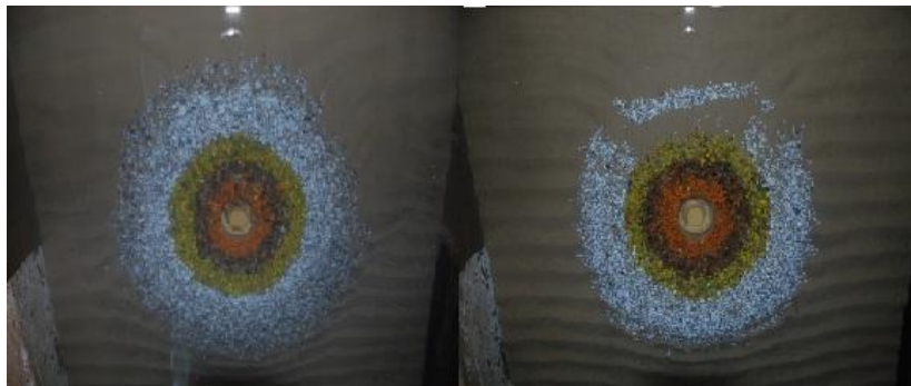
Figure 4.33 – Left: test s1_001 statically stable with less deposition at the downstream side. Right: test s1_002 with downstream deposition at the white ring. Flow direction from the bottom to the top.
