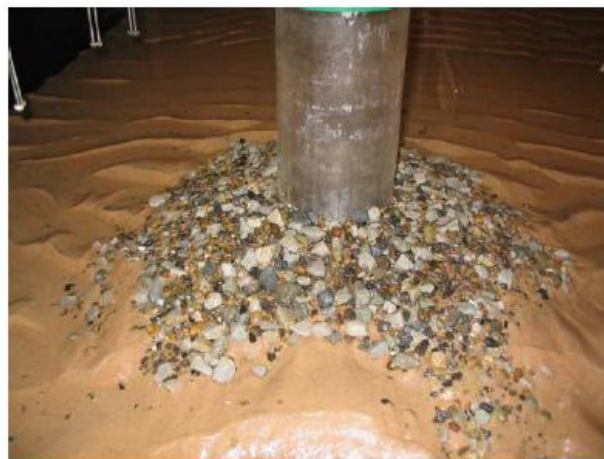
Figure 3.32 – Physical model of a damaged scour protection around a monopile from [169].
