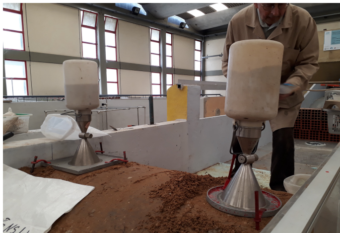
Sand replacement test
