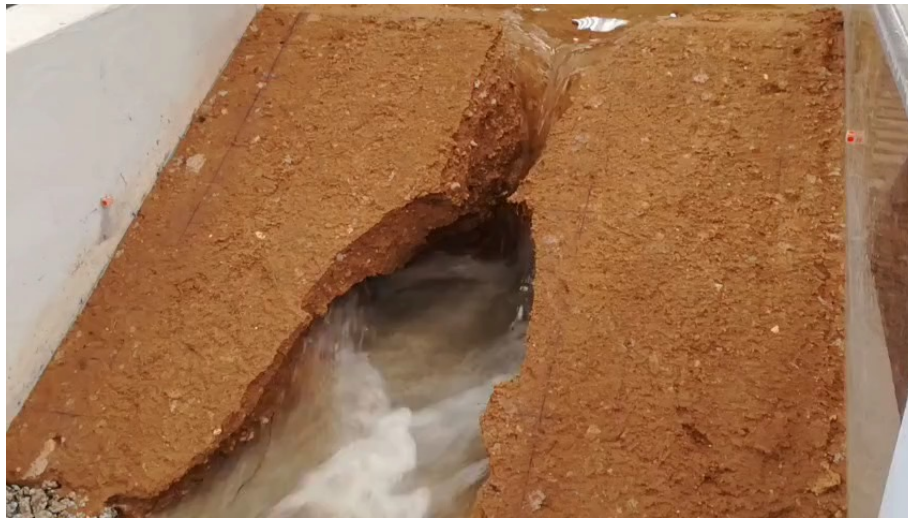
Test 1: Homogeneous dam with toe drain
