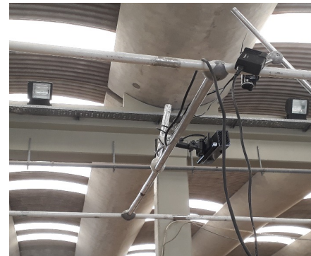
KINECT sensor and video camera above the crest
