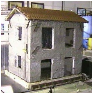
Building 1 (B1) 2-storey prototype building (EUCENTRE experimental campaign) (Penna 2015)
