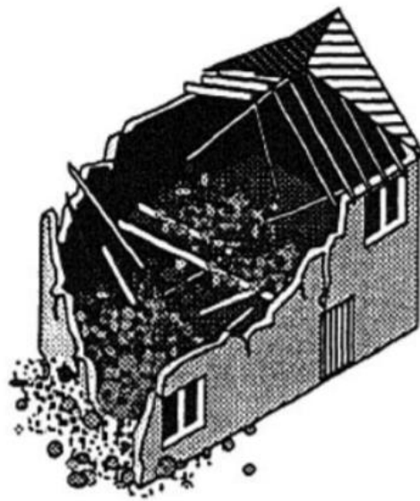
Damage Level: D5 Collapse Extent of Collapse: 50% of Volume
