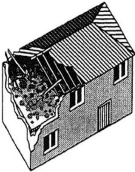
Damage Level: D5 Collapse Extent of Collapse: 10% of Volume
