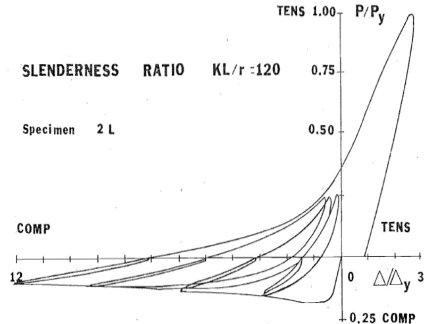
Hysteretic Behavior of Bracing members and seismic response of braced frames with different proportions. A.K. Jain, S.C.Goel ,R.D.Hanson , Report no. UMEE 78R3 , 1978.
