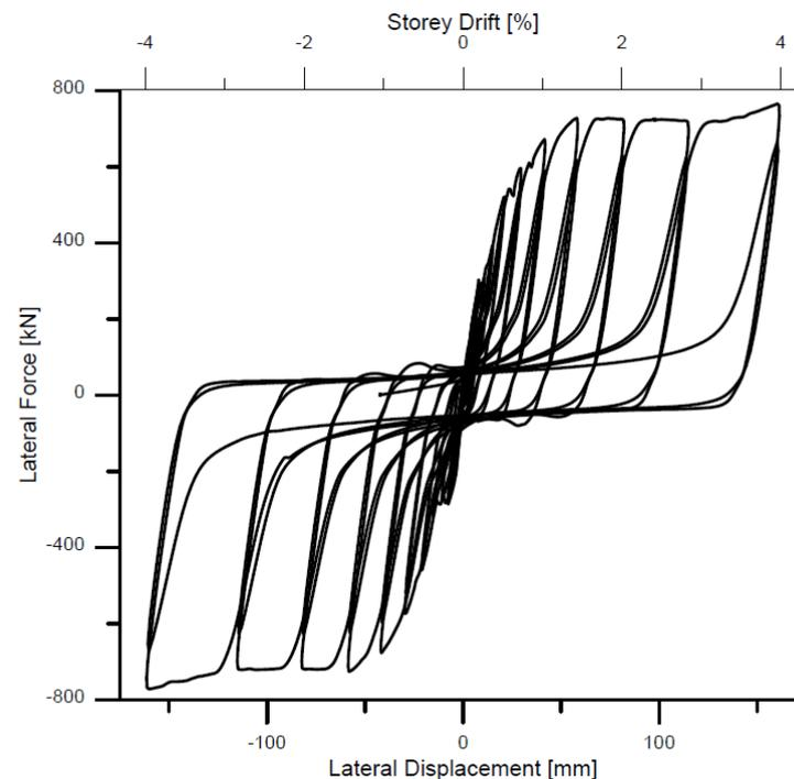
Figure 3-66: Lateral force vs. displacement hysteretic performance of plain cross brace sample
