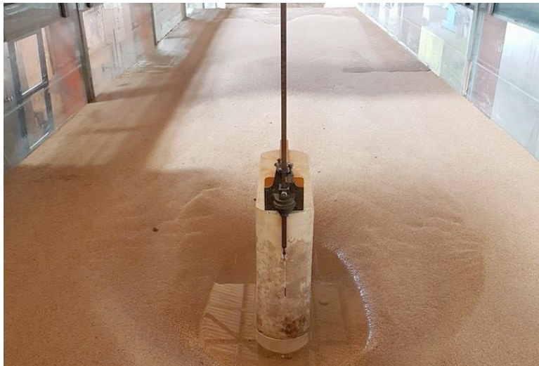
Scour hole at pier vicinity ( W = 14 cm; d_s = 23 cm - 3 days)
