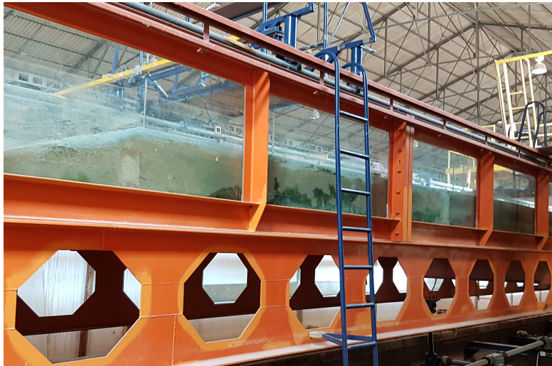
Flume at LNEC (40 m long and 2 m wide)
