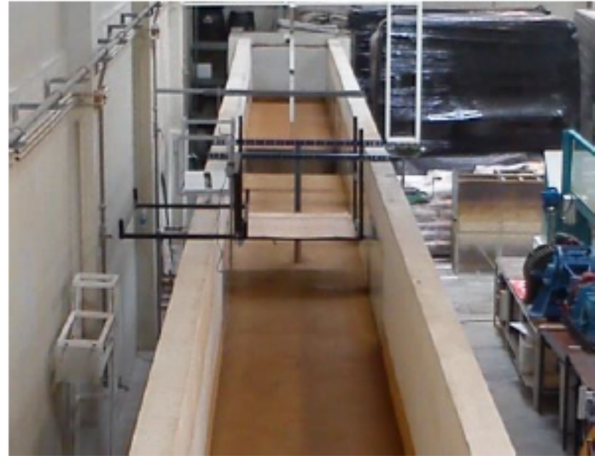
Flume at FEUP (32.2 long and 1 m wide)
