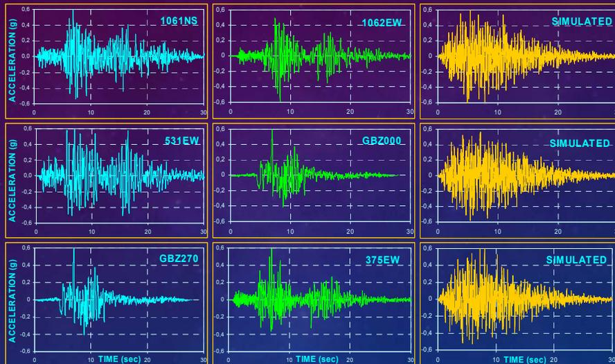
Two sets of scaled real and one set of simulated acceleration records
