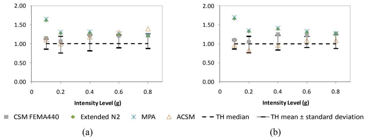
Fig. 4. Top displacement ratios, centre of mass (a) X direction; (b) Y direction.
