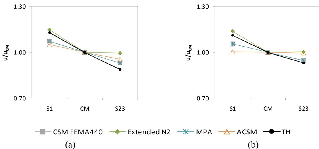
Fig. 7. Normalized top displacements X direction (a) 0.2g; (b) 0.6g.
