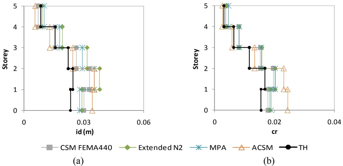
Fig. 6. X direction (a) Interstorey drifts profile (m), column S23, 0.4g; (b) Chord rotations profile, column S13, 0.6g.
