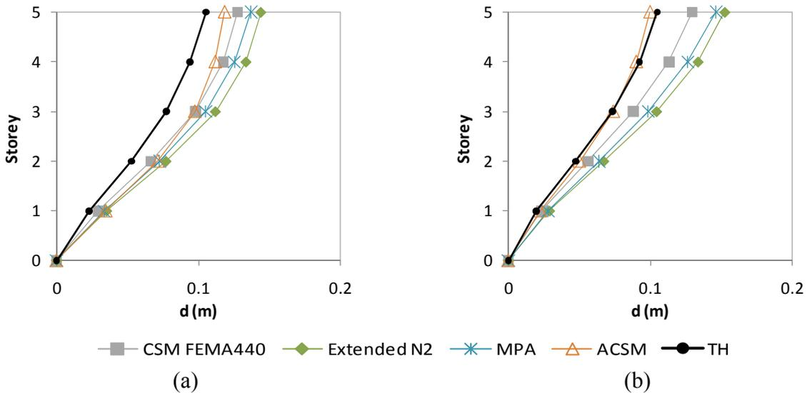
Fig. 5. Lateral displacement profile (m), column S1, 0.4g (a) X direction; (b) Y direction.
