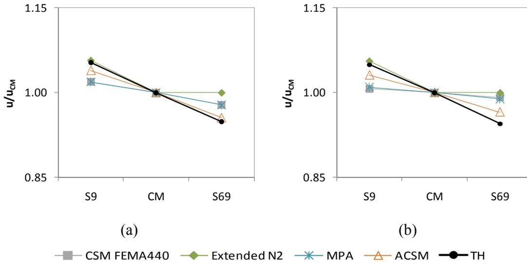
Fig. 11. Normalized top displacements, X direction a) 0.2g; b) 0.4g.
