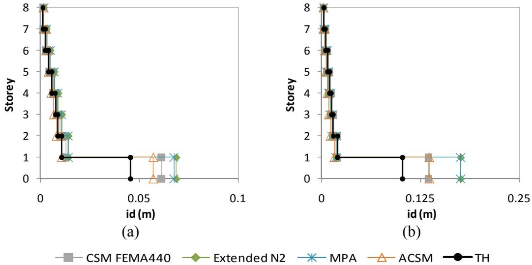
Fig. 10. Interstorey drifts profiles X direction a) Column S72, 0.2g; b) Column S52, 0.4g.
