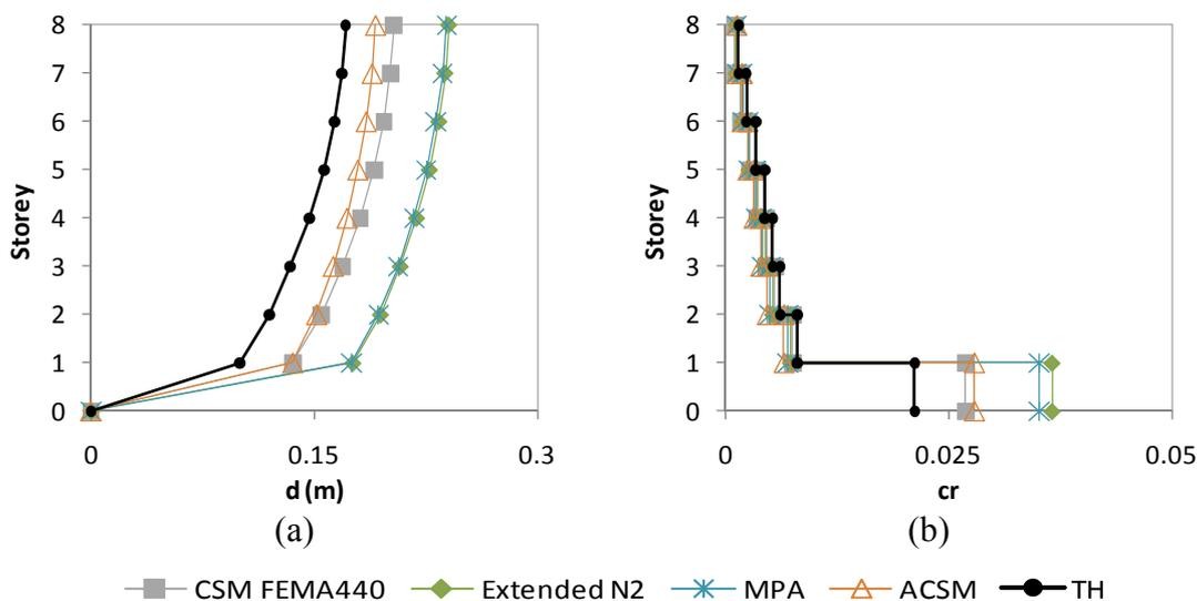
Fig. 9. X direction a) Lateral displacement profile (m), column S69, 0.4g; b) Chord rotations profile, column S9, 0.4g.
