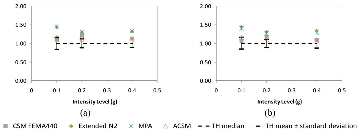
Fig. 8. Top displacements ratios, X direction a) centre of mass; b) column S9.
