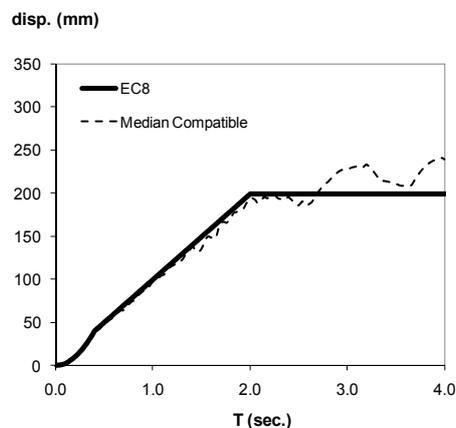
Fig. 3. Displacement response spectra, 0.4g.
