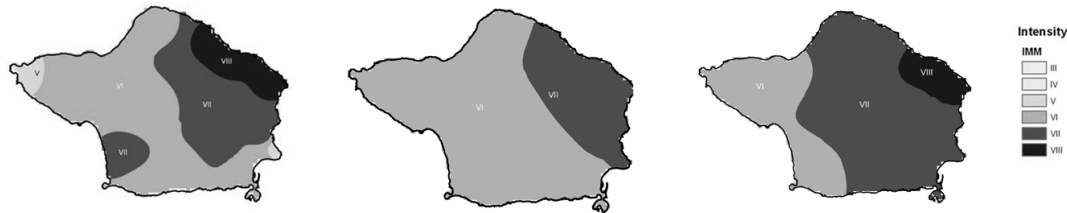
Figure 10: Left to right panels: MMI maps derived from (1) surveyed data (from Matias et al. , 2007), computed using the conversion PGA -MMI (Wald et al. , 1999), (2) for EPI1 and (3) for EPI2. The isoseismal maps were drawn using the ArcGIS interpolation Inverse Distance Weight method (IDW)
