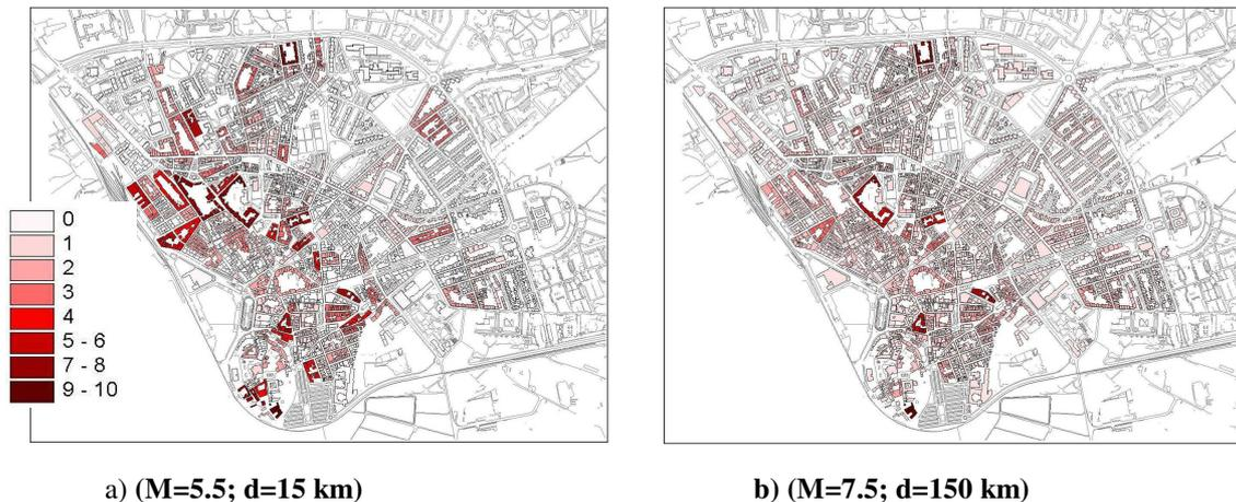
Figure 8 - Damage scenarios by the block (*method 1*). (Number of buildings which collapse per block).
