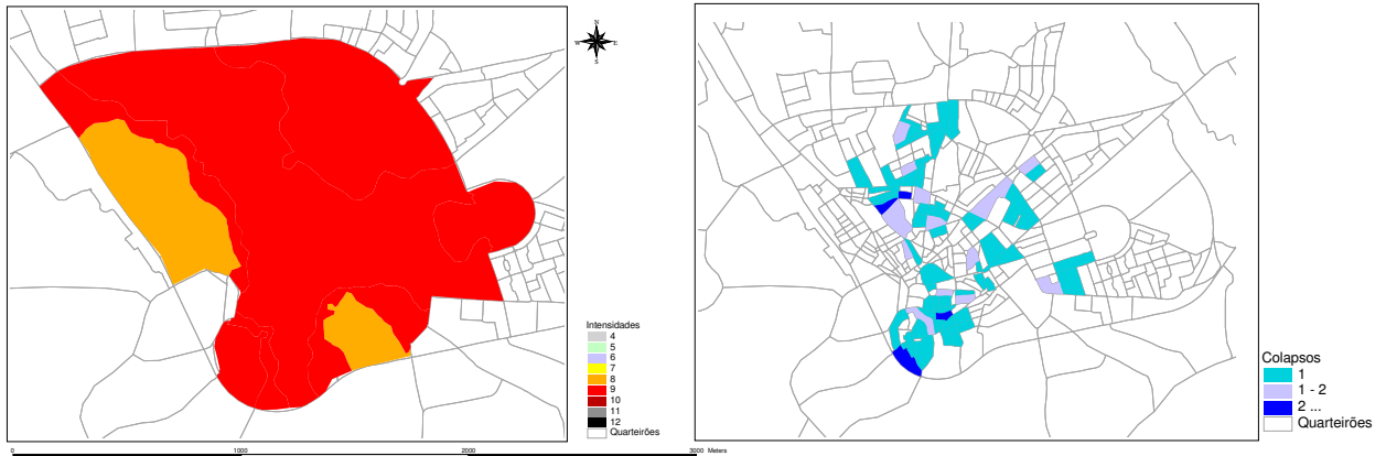
Figure 28 - Intensities and damage for the 1755 earthquake – distant scenario M=8.75 R=200 km
