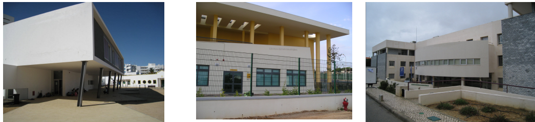
Figure 5. Example of some factors able to modify seismic behaviour; left– soft-storey; centre – setbacks; right – plan asymmetry.
