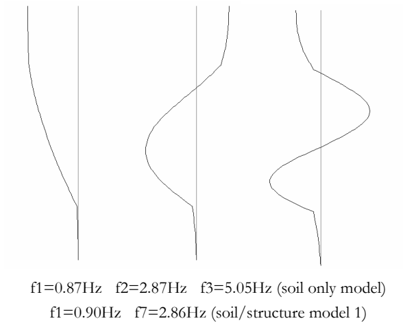
Figure 2.13 – Soil only modes of vibration in cantilever model
