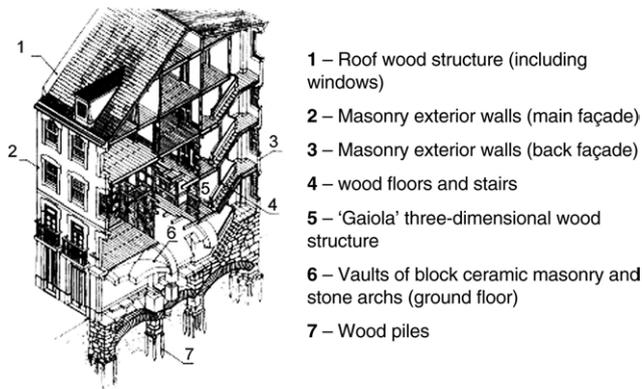
Fig. 1. Structural details of a 'Pombalino' building (adapted from [2]).
