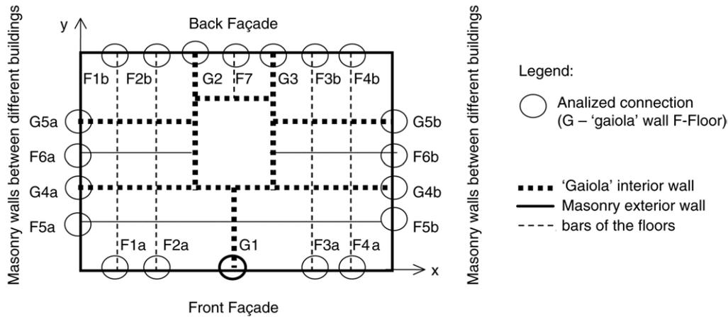
Fig. 10. Analysed connections between timber elements and masonry walls.
