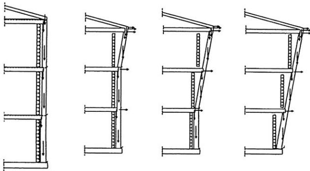
Fig. 12. Bending out-of-plane of masonry buildings as a typical collapse mechanism due to seismic actions [12].
