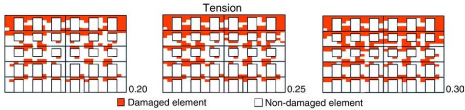
Fig. 11. Damage levels in masonry elements from main façade for increasing values of  $\gamma_{sis}$ .
