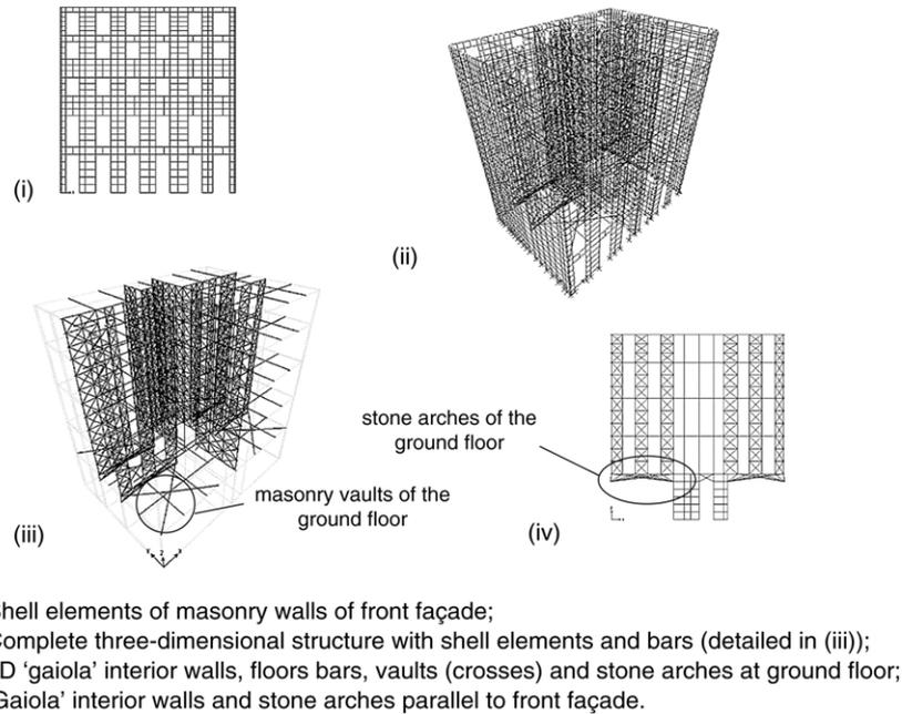
Fig. 7. Numerical model of the building [7].
