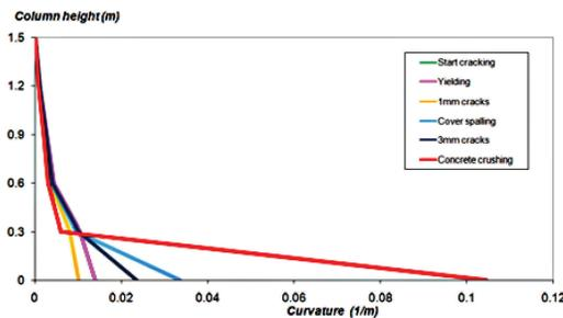
Figure 2. Section curvatures values along the column for various damage state (axial force ratio  $n = 0.4$ ).
