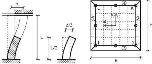
Figure 1. Column model and transverse section modelling.
