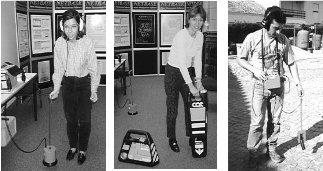
Figure 8 - Ground microphone (indirect acoustic sounding)
