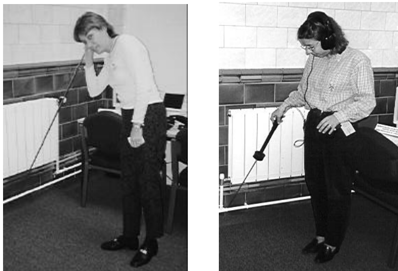
Figure 7 - Acoustic and electric stethoscope (direct acoustic sounding)
