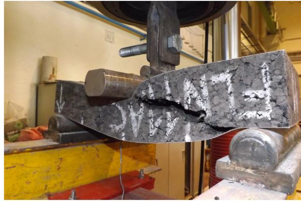
Fig. 9. (a) Results from testing of specimens CS1–CS5 and (b) typical collapse mode in tests on specimens CS1–CS5.
