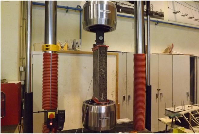
Fig. 4. Setup for the edgewise test.
