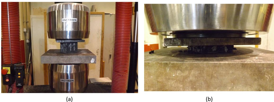
**Fig. 2.** Unloaded specimen (a) and fully loaded specimen (b).
