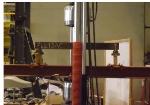
Fig. 10. Setup for the tests for evaluation of flexural and shear stiffness of specimens composed of CA core and GFRP facings.
