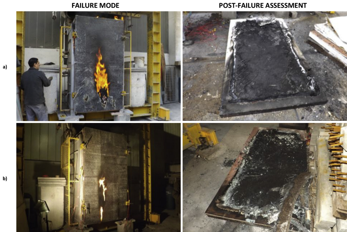
Fig. 7. Failure mode and post-failure assessment of CA core wall assemblies: (a) P-CA; (b) P-CA-FG.
