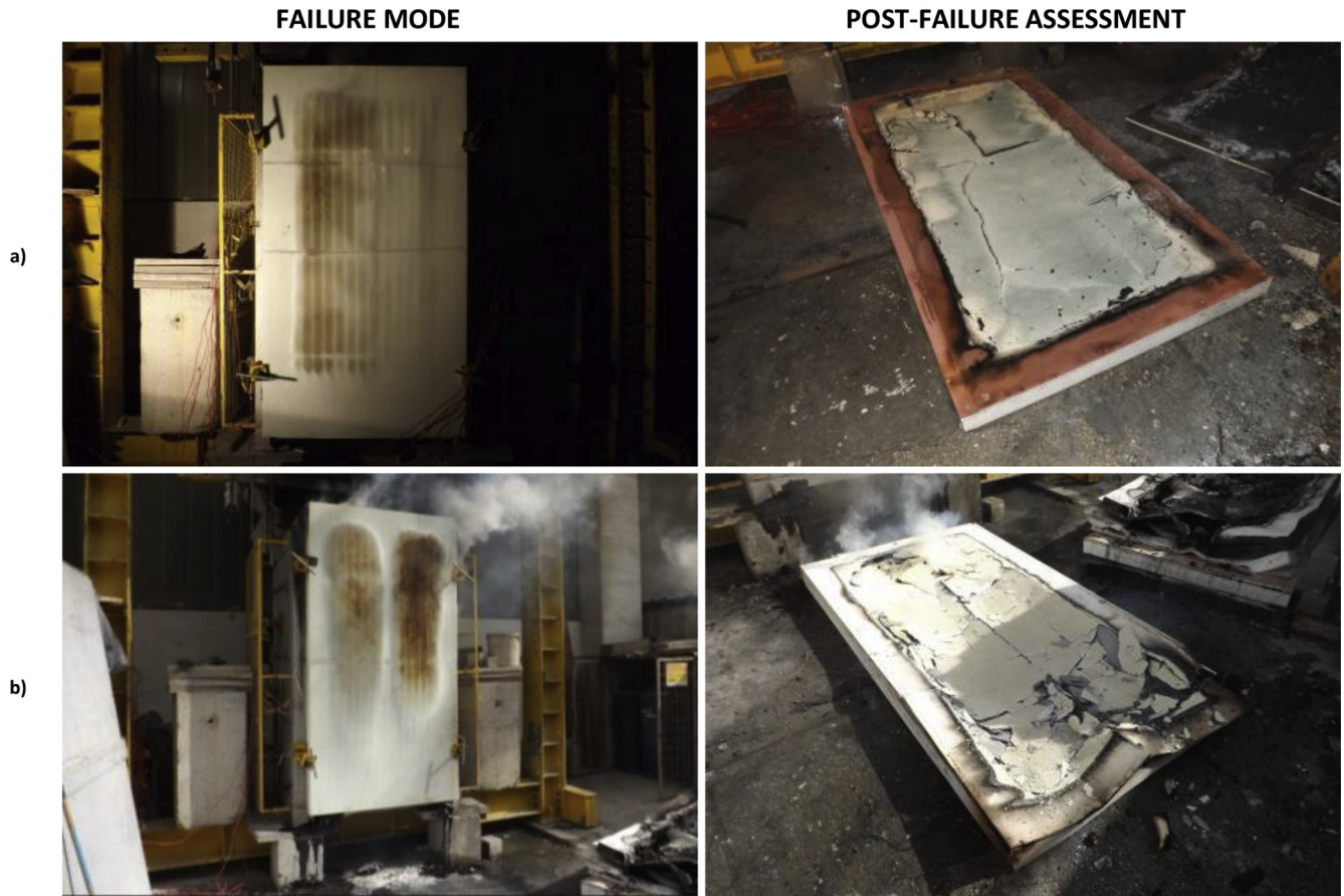
Fig. 6. Failure mode and post-fire assessment of PET foam core wall assemblies: (a) P-PET-FG; (b) P-PET-MGO/HS.
