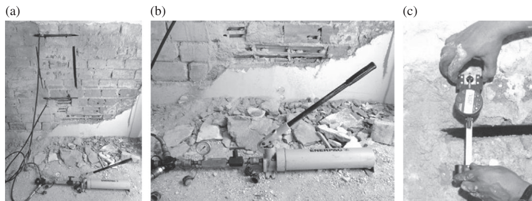
Figure 3 Test apparatus: (a) test setup; (b) hydraulic pump; and (c) removable mechanical meter.
