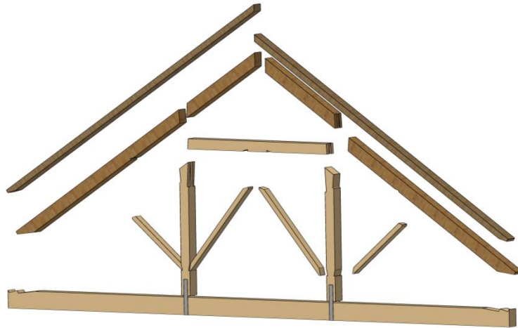
Figure 6. São Roque Church: Exploded view of the truss.
