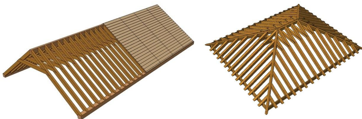
Figure 1. Traditional Portuguese rafter roofs, gabled and hipped.
