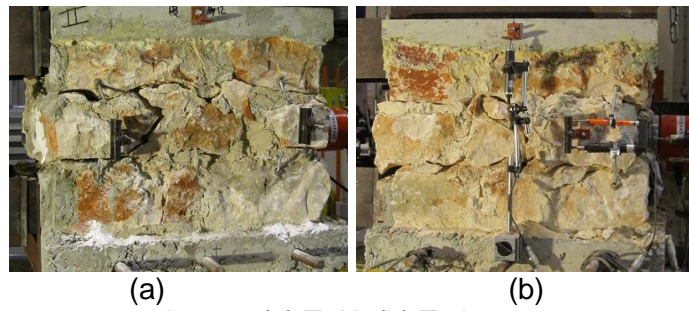
Figure 8. Crack pattern of masonry specimens: (a) T1H, (b) T7A
