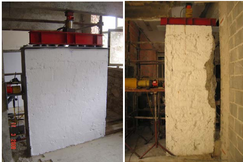
Figure 3.1 Test setup (left) and general view of a concrete block specimen (centre) and of a rubble stone specimen (right)
