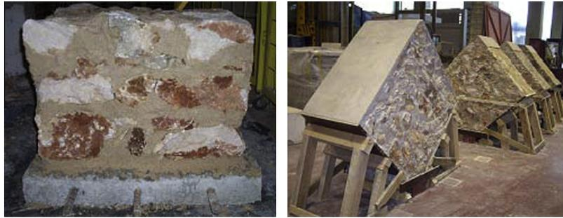
Fig. 1. View of a triplet test specimen with three horizontal layers (left) and of diagonal compression test specimens (right).
