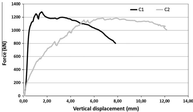
Fig. 2. Compression tests – “force–displacement” diagrams.
