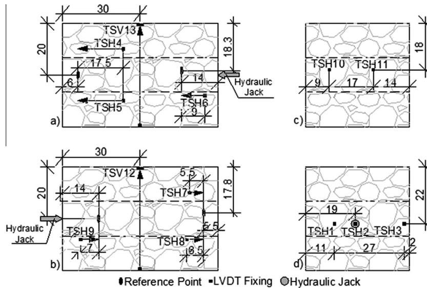
**Fig. 4.** Triplet tests – transducers on the specimen’s front (a) and back (b) faces, on the restrained lateral face (c) and on the loaded lateral face (d) (dimensions in (cm)).
