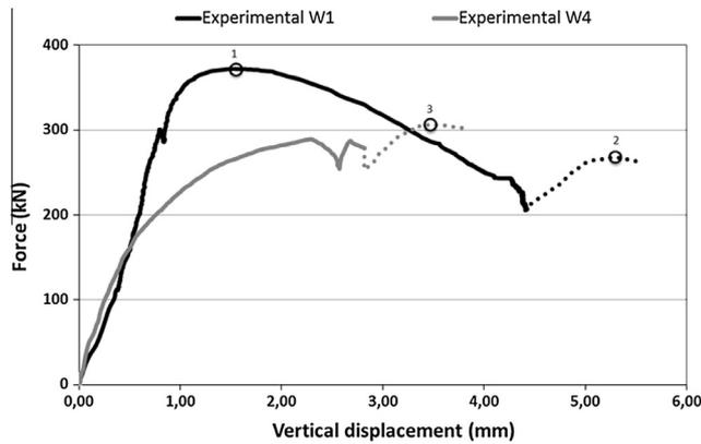
Fig. 14. Diagonal compression tests – “force–displacement” diagrams for hydraulic lime mortar specimens.
