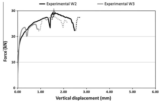
Fig. 15. Diagonal compression tests – “force–displacement” diagrams for air lime mortar specimens.
