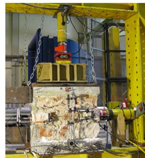
Fig. 3. Setup for triplet test.
