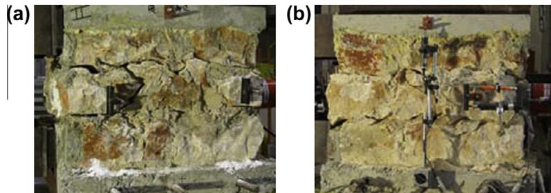
**Fig. 5.** Crack pattern of masonry specimens: (a) specimen T1 and (b) specimen T7.
