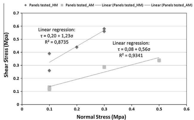
Fig. 11. Triplet tests – relation between shear stress and normal stress for hydraulic and air lime mortar specimens ( $R$  is correlation coefficient of the linear regression).
