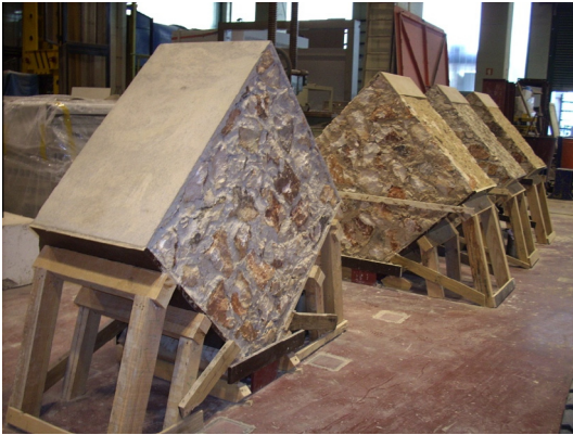
Fig. 1. Panels for diagonal compression tests.
