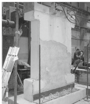
(b) CFRP reinforced render detachment (EPF_06 specimen)
