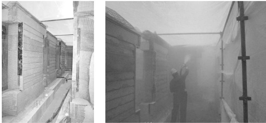
Fig. 2. Masonry wall specimens (left) and render mortar shotcrete operation (right).
