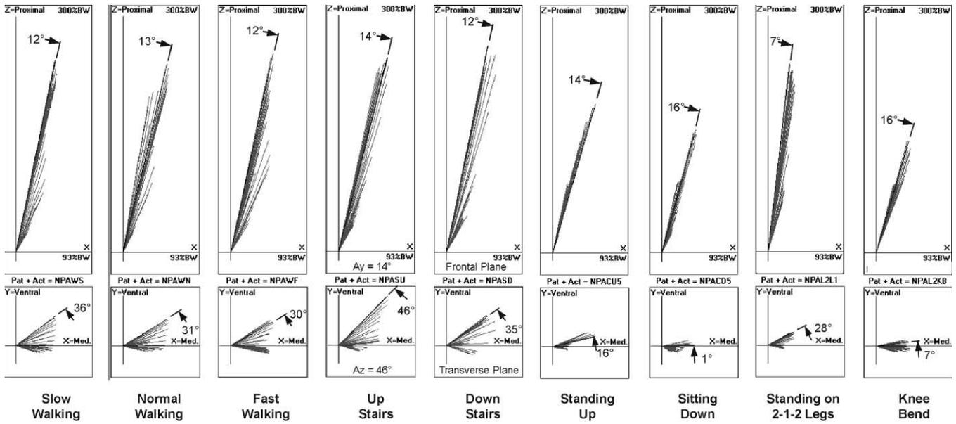
Fig. 8. Contact force vector  $F$  of typical patient NPA during nine activities. The  $z$ -scales go up to 300% BW. *Upper diagrams*: Force vector  $F$  and direction  $A_y$  of  $F$  in the frontal plane. *Lower diagrams*: Force vector  $F$  and direction  $A_z$  of  $F$  in the transverse plane.
