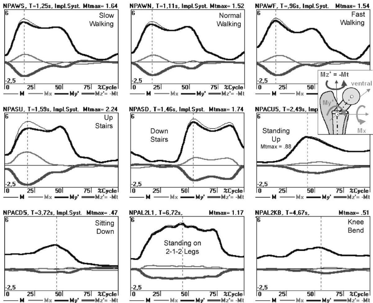
Fig. 9. Implant moment  $M$  of typical patient NPA during nine activities. Implant moment  $M$  and its components  $M_x, M_y, M_z = -M_t$  in % BW m.  $M$  and  $M_z$  are nearly identical. The scale range is  $-2.5-6\%$  BW m. Negative  $M_z$  cause inwards torsion around the implant stem. Cycle duration  $T$  and peak torsional moment  $M_{tp} = M_{tmax} = -M_{zp}$  are indicated in diagrams.
