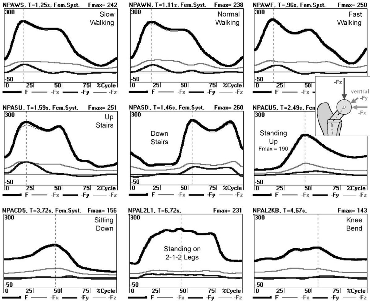
Fig. 6. Contact force  $F$  of typical patient NPA during nine activities. Contact force  $F$  and its components  $-F_x$ ,  $-F_y$ ,  $-F_z$ .  $F$  and  $-F_z$  are nearly identical. The scale range is  $-50$ – $300\%$  BW. Cycle duration and peak force  $F_p = F_{max}$  are indicated in diagrams.
