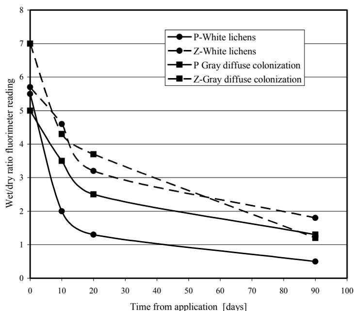
**Figure 3:** The wet/dry ratio of the fluorimeter readings for three successive applications of biocide solutions at 1.5 % concentrations for the case of white lichens and gray diffuse colonization. Key: P indicates Preventol, Z indicates zinc chloride solution
