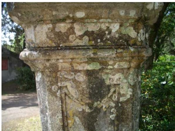
**Figure 4:** Detail of the area of the pedestal where the left half was treated with a 2 % Preventol solution and the right half with the 2 % zinc chloride solution. Only one application was used. The stone has been wetted for the measurements and this highlights the active biocolonization which tends to look greener when wet.
