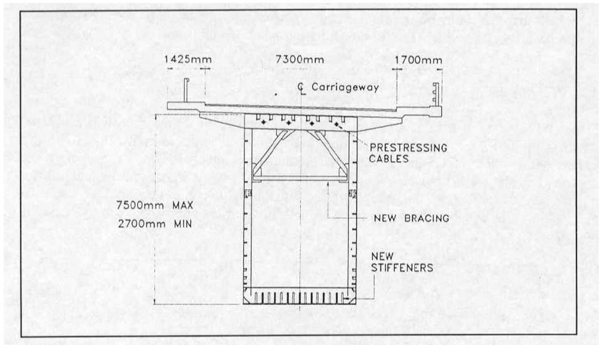
Figure A.8 Main strengthening details (Slater 1997).
