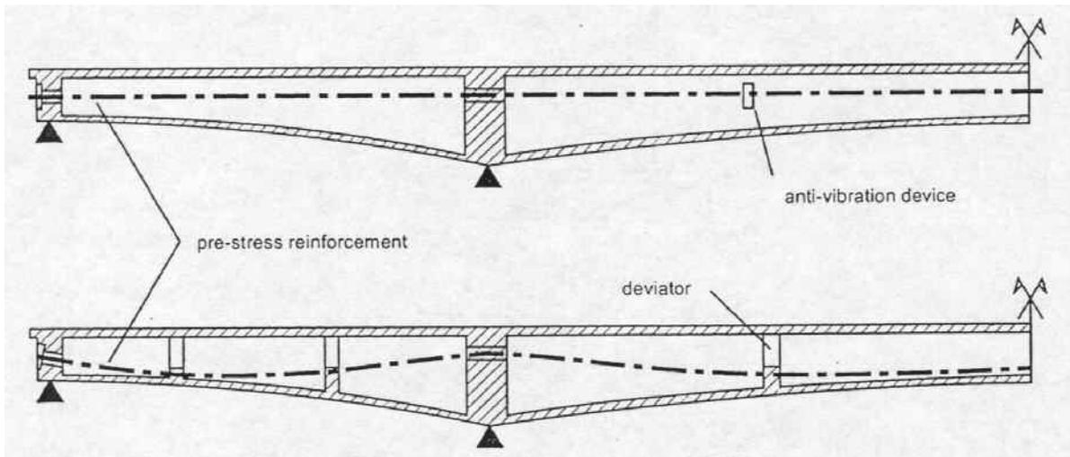
**Figure 2 Tendon profiles for box girder.**
