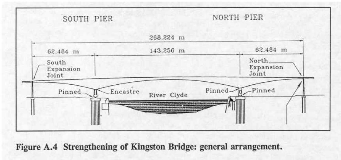
Figure A.4 Strengthening of Kingston Bridge: general arrangement.
