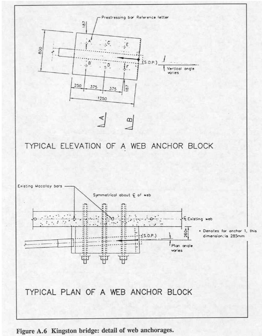
Figure A.6 Kingston bridge: detail of web anchorages.
