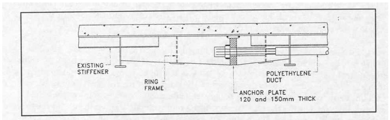
Figure A.9 Anchorage detail (Slater 1997).
