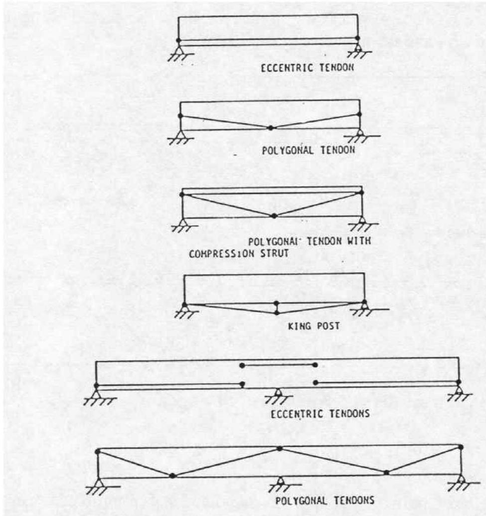
Figure 1 Different tendon configurations (from Xanthakos 1996)
