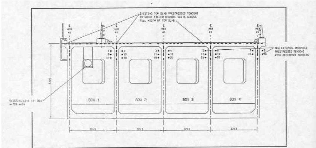
Figure A.2 Clifton Bridge strengthening: position of tendons.
