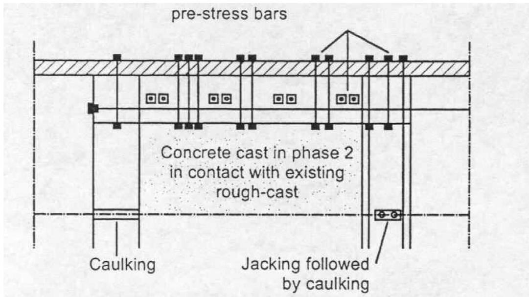
**Figure 5 Anchor block attached using a series of ties.**
