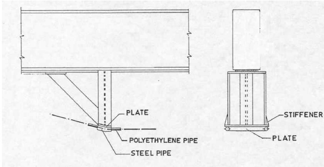
Figure 9 Deviator to increase cable eccentricity below bottom flange.
