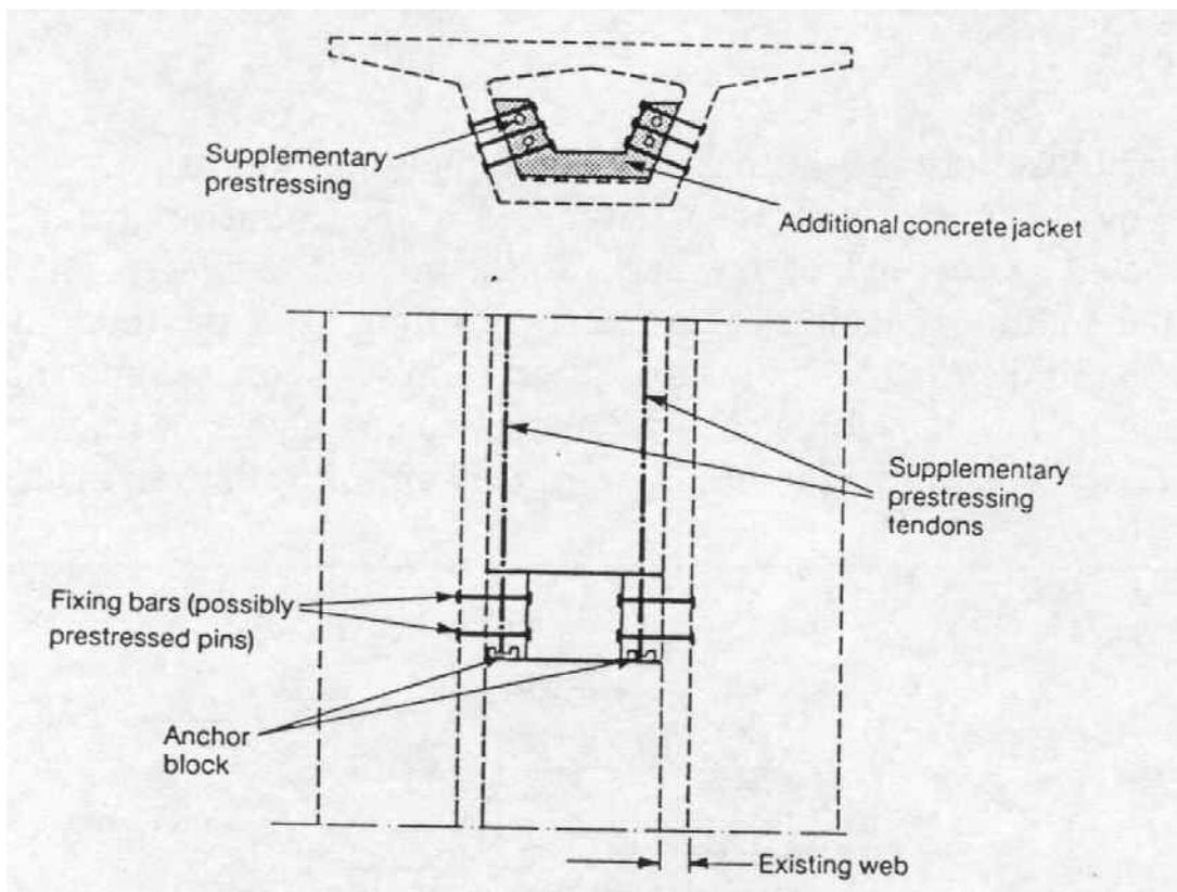
**Figure 4 Bonded anchor block using in-situ concrete.**
