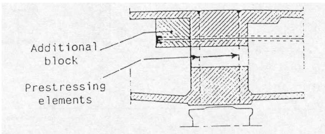
**Figure 6 Diaphragm anchoring.**
