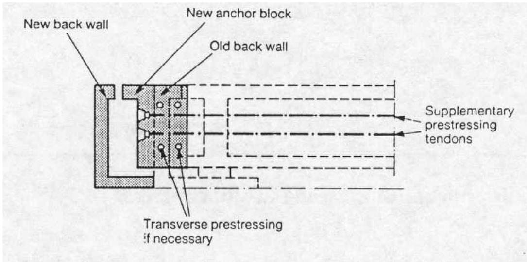
**Figure 3 End anchor block.**
