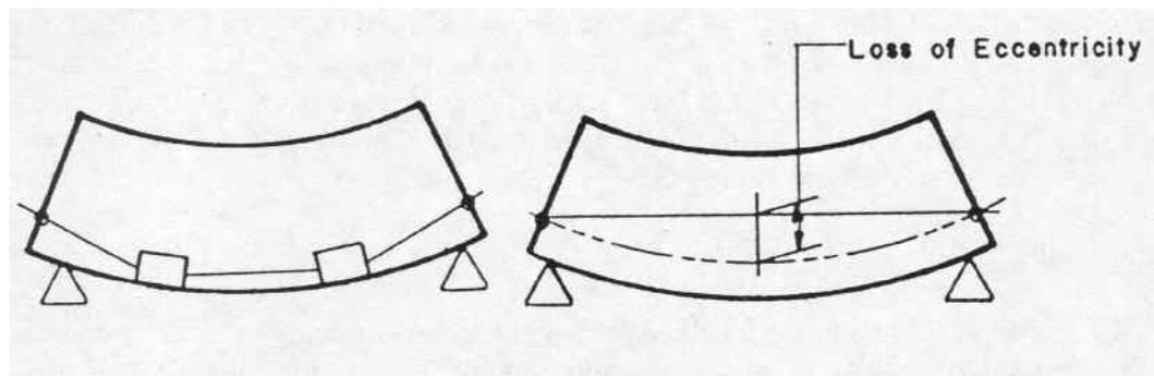
Figure 10 Distribution of deviators to prevent loss of eccentricity (from Muller and Gauthier, SP-120).
