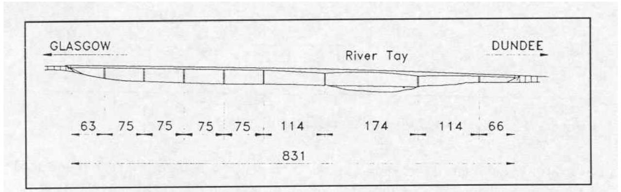
Figure A.7 General elevation of Friarton Bridge.
